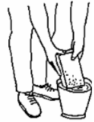
Wet the bricks before laying them
