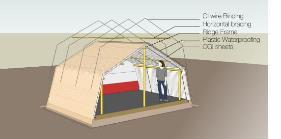
**Step 5** : Tie purlins of wood/bamboo as shown in figure above. Then lay the CGI sheets and then Plastic waterproofing. Tie horizontal bracings with purlins below the CGI sheets. Then the tie whole roofing with the pipes inserted to the ground with 3 fold GI wire.
