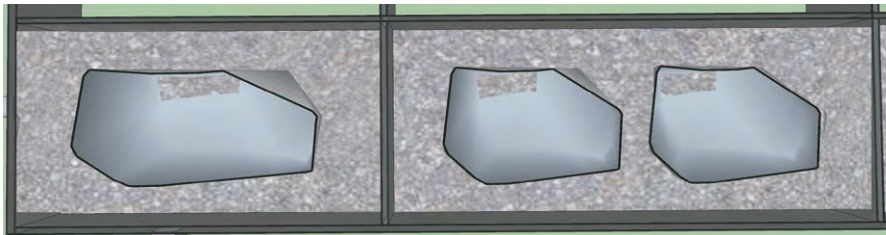
Plan view: Stone in the middle with 1” gaps on the side and middle.
