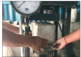
3. Compressive strength test by universal testing machine
